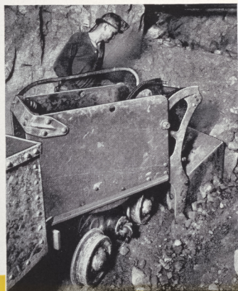
Model 12 Eimco-Finlay Loader in operation at the largest copper-producing property in Montana. Note how easily bucket crowds into muck. Recent repeat orders have brought the present number of Eimco-Finlay Loaders at this famous property up to twenty-three.
